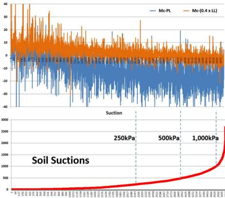
The base line (red) plots the soil suction test results. The orange line plots data using 0.4 x LL and the blue line the Mc compared with the PL. Although there is very broad agreement, the amplitude of desiccation is best revealed by the suction test - both comparisons with the PI tests show increasing desiccation in a linear fashion and there is substantial scatter which renders them less reliable than the suction test.
